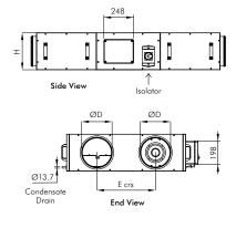
The CLASSIC 330 unit is optimised for an y commercial building services application covering an airflow envelope of 0. 156 - 0.383m<sup>3</sup>/s at 75Pa ESP (low pressure duct systems). Overall unit SFP calculated with F7 / M5 filters under clean filter conditions.
